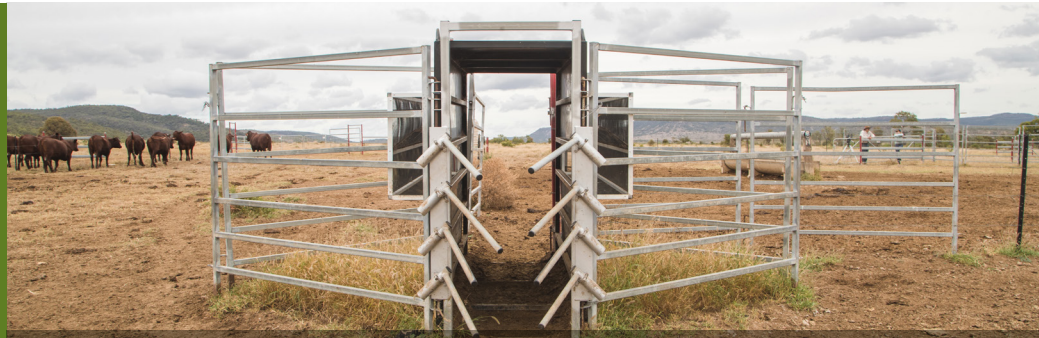
Pictured: one of the three Walk Over Weigh (WOW) units installed for this trial. WOW units identify and record the liveweight of cattle each time they pass through. This data combined with satellite pasture data make up the Remote Livestock Management System (RLMS).
