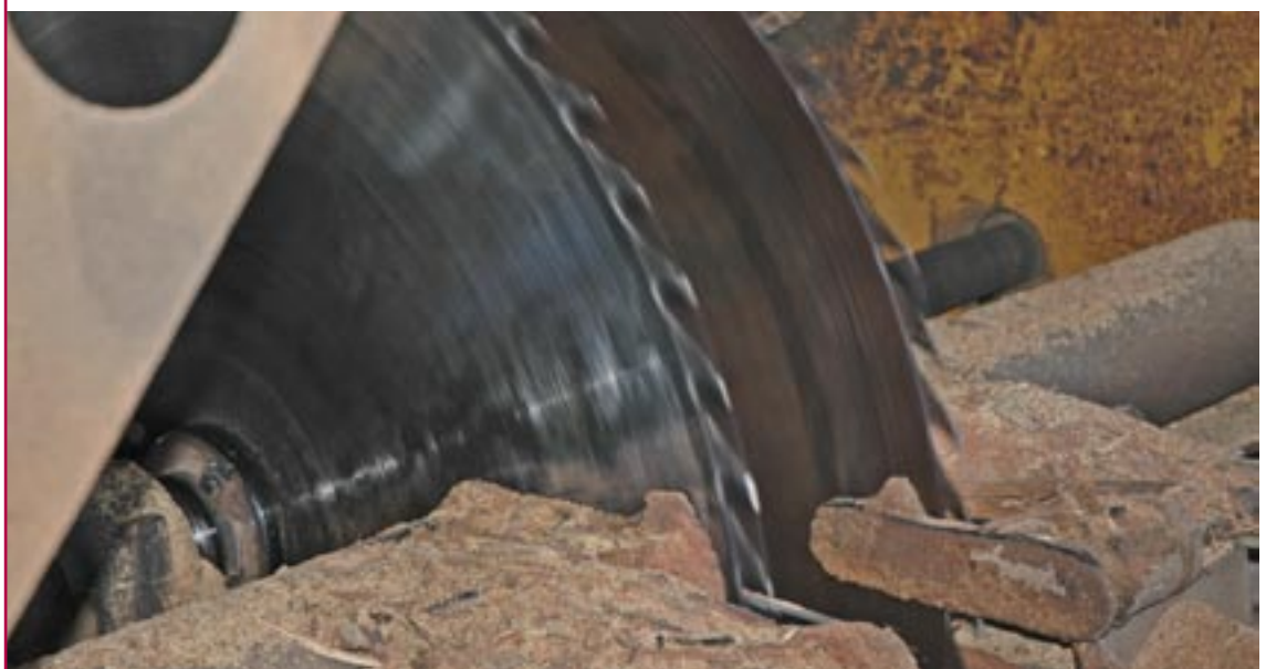
6 inch twin edger used for cutting mining timber
