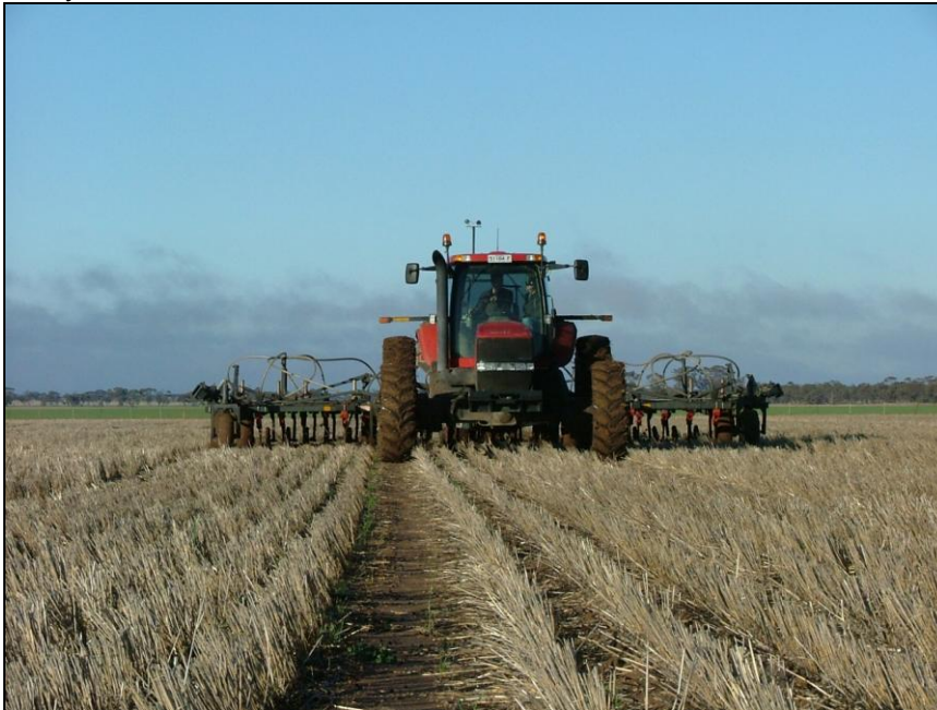
Figure 6: CTF system – defined wheel tracks. Source: Tim Neale, CTF Solutions
