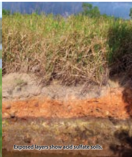
Any deep excavation may disturb and expose the dark grey and wet acid sulfate soils
