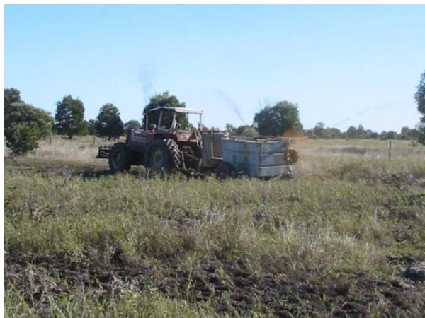
Figure 6: Compost tea being applied using a customised spray rig. A front tank contains the food and nutrient sources while the rear tank contains the tea/extract. Products remain separated until they converge at the boomless jet.
